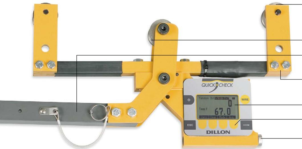
Sheaves with bearings eliminate friction and provide the best accuracy
